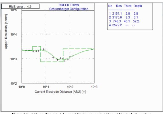
Figure 3.0: A Curve (Graph) of Apparent Resistivity against Current Electrode Separation
